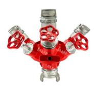
The **Tri-Valve Fire Division**, also known as the Three-Valve Division, is an essential piece of equipment for fire-fighting water systems. It allows a main water line to be divided into three separate outlets, facilitating the intervention of rescue teams. Available in **PN 25 and PN 16**, this tri-division ensures smooth, safe distribution of water flow, guaranteeing optimum performance.
